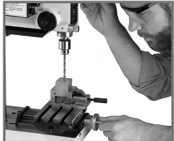
Figure 11. Wear eye protection and secure-ly clamp workpiece when operating mill.
